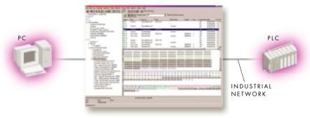
As industrial networks become increasingly mission-critical, the cost of downtime can be thousands of dollars per hour, and undetected, underperforming networks can further cut profitability. Locating the cause of poor performance can take hours, or days. Communications analyzers provide a view inside the network traffic, enabling administrators to locate the root cause and quickly take corrective action  $\blacktriangle$
